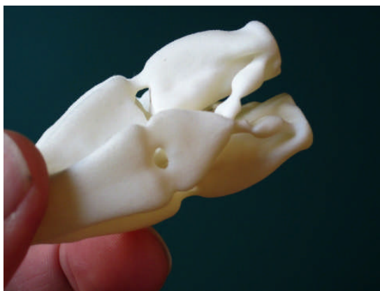
Figure 1: Complex alternated gripper. This complex 3D compliant mechanism was designed with topology optimization and produced using additive manufacturing.
