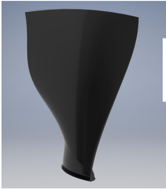
Figure 9.1: Rendered CAD model of optimised fan blade
