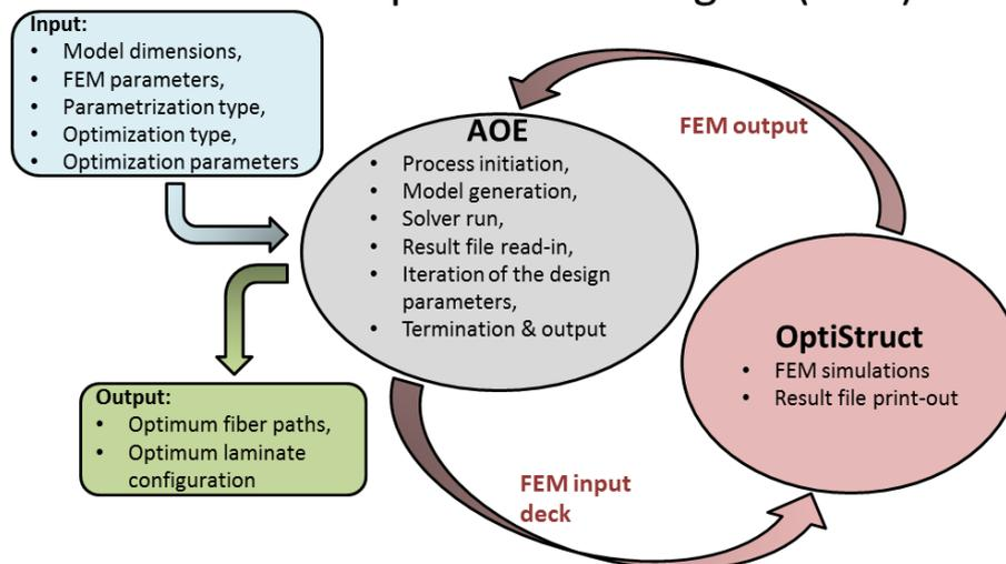
Figure 13.1: A schematic diagram showing the working principle of AOE.
