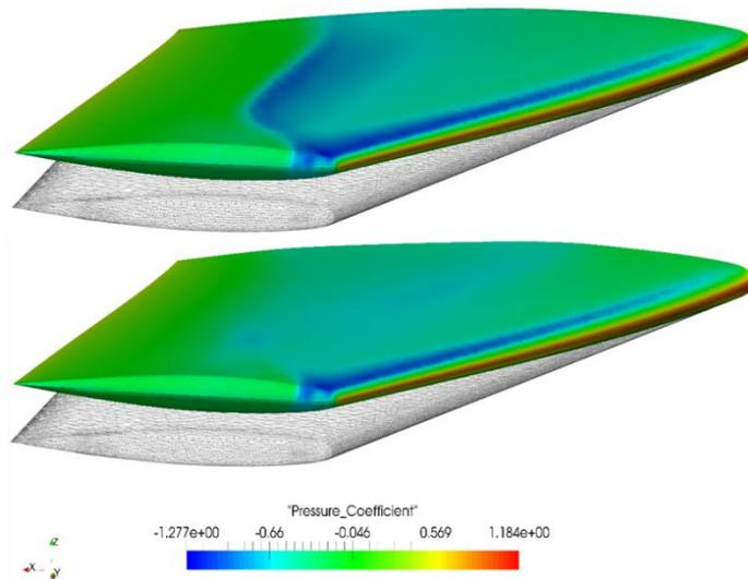
**Figure 2.6: Initial (top) and optimized (bottom) pressure distribution at a flexible ONERA M6 wing. Black indicates the jig-shape. Results correspond to some 30% improved drag at constrained lift and thickness each in the deflected state.**
