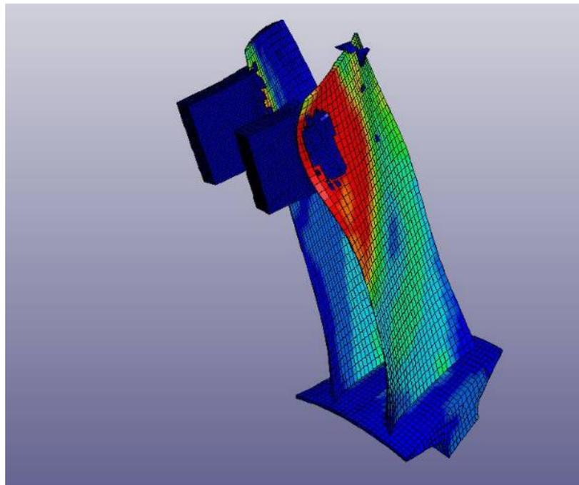
**Figure 8.1: Ice impact model with two impacting ice slaps onto two disks.**
