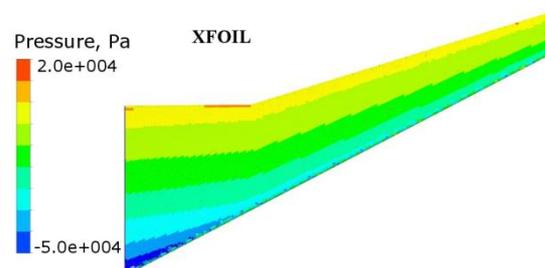
Figure 3.2: Pressure distribution for a wing obtained by ANSYS Fluent (left), XFOIL software (right).
