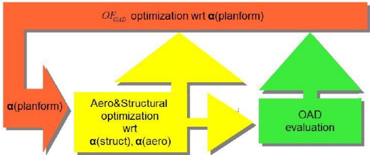
**Figure 6.2: Overall Aircraft Design top level optimisation on top of the aero-elastic and structural ones;  $\alpha(\text{struct})$  and  $\alpha(\text{aero})$  are the structural and aerodynamic variables respectively.**
