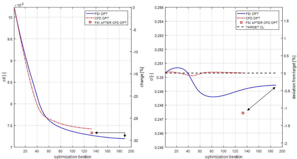
**Figure 2.7: Comparison of a single disciplinary (CFD) and multidisciplinary (aeroelastic / FSI) node-based shape optimisation of the ONERA M6. Left diagram shows the drag coefficient as objective function and the right diagram shows the lift coefficient as constraint. Note that the FSI optimisation performs better in both cases.**
