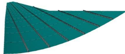
Figure 3.1: Ribs and spars definition (a), stringer components and its possible shape (b)
