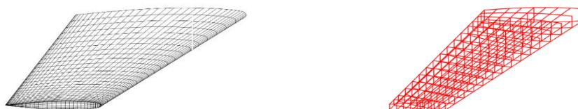
**Figure 5.1: Structured CFD model (left) and a structural Nastran-based model (right) of an ONERA M6 wing. Courtesy of ONERA.**
