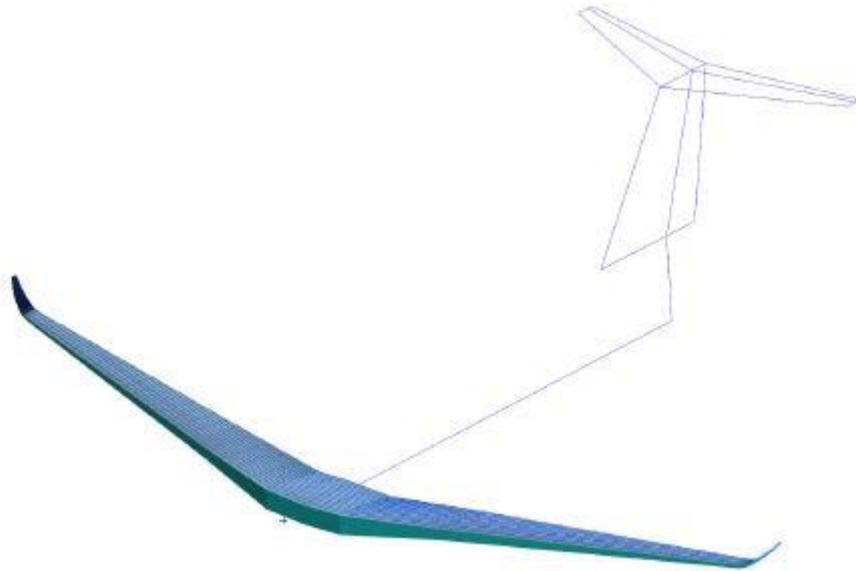
**Figure 12.1: Aircraft wing model used in the optimisation.**
