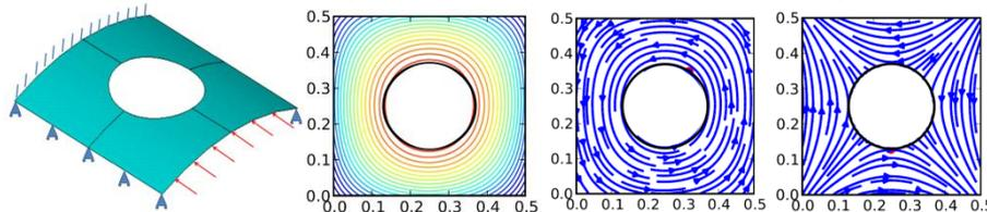
Figure 3.7: Problem example (left), optimal iso-lines obtained by 9 parameters (middle), optimal fibres placement for  $[\pm\alpha]_s$  laminate with MFCC =  $10 \text{ m}^{-1}$  at each layer of laminate (right)
