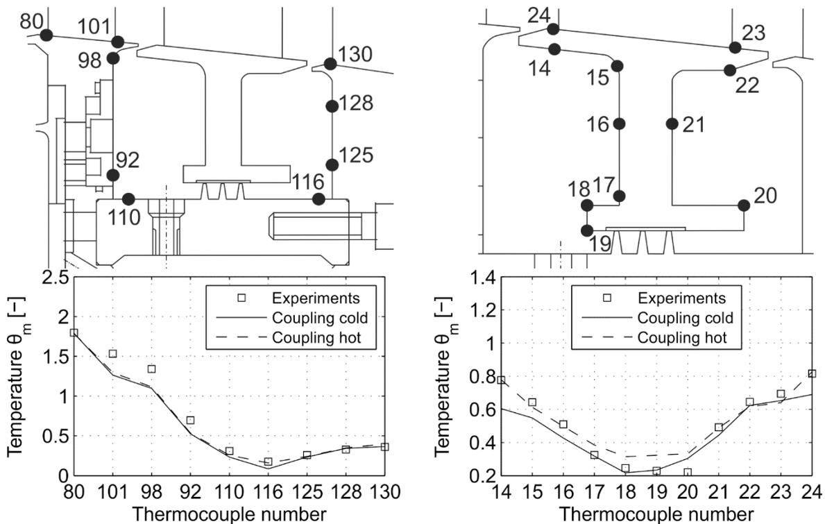
**Figure 7.4: Rotor (left) and stator (right) disc.**
