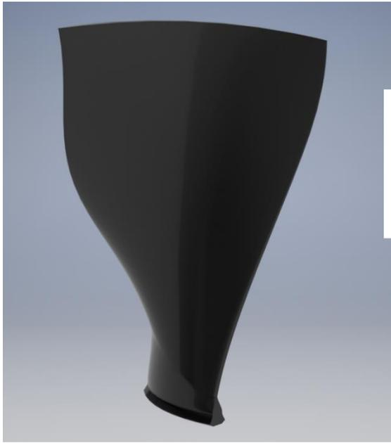
**Figure 9.1: Rendered CAD model of optimised fan blade**
