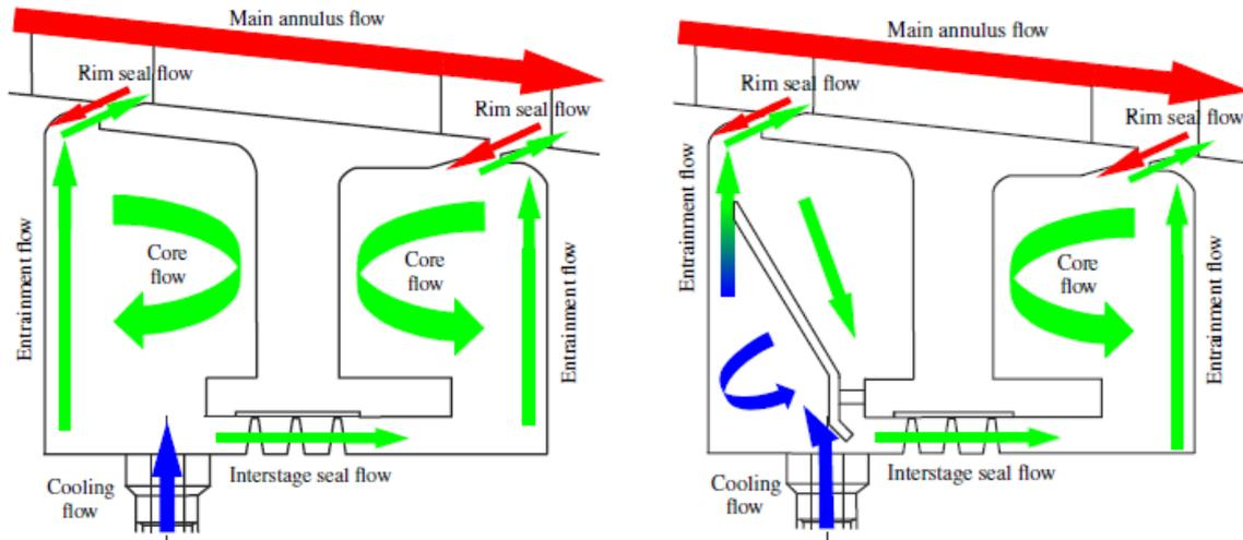
**Figure 7.3: Turbine Stator well flow structure for standard geometry (left), with inserted deflector (right).**
