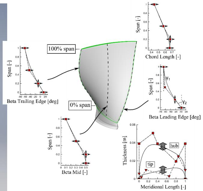
**Figure 9.2: Fan blade parametrisation**
